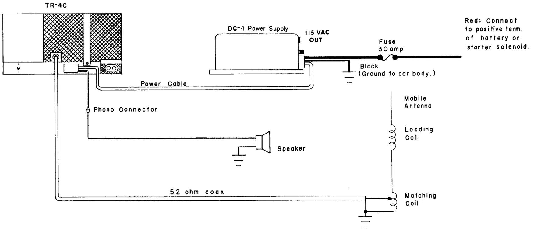
Figure 2-3. Electrical Connections Required for Mobile Installation
