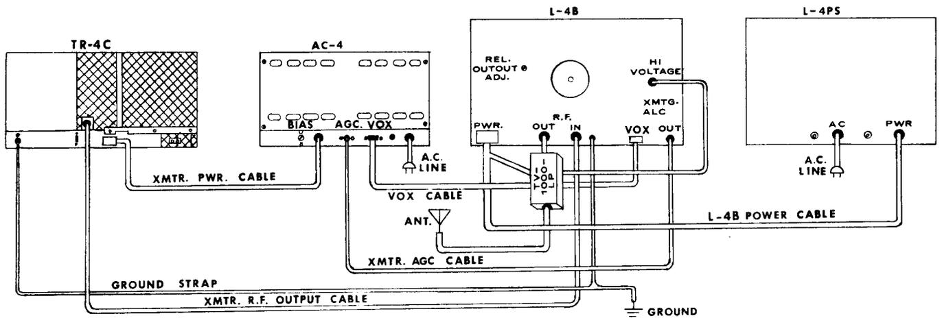
Figure 2-8. Connecting the AC-4 Power Supply and the L-4B Linear Amplifier
