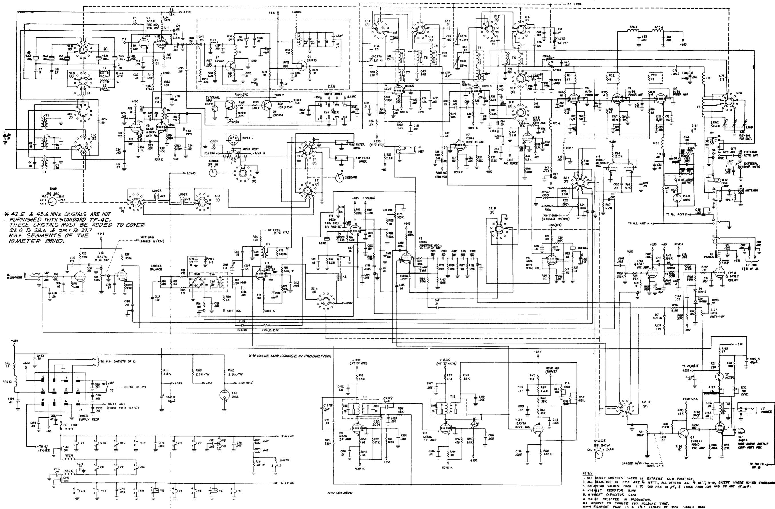
Figure 5-5. TR-4C Schematic
