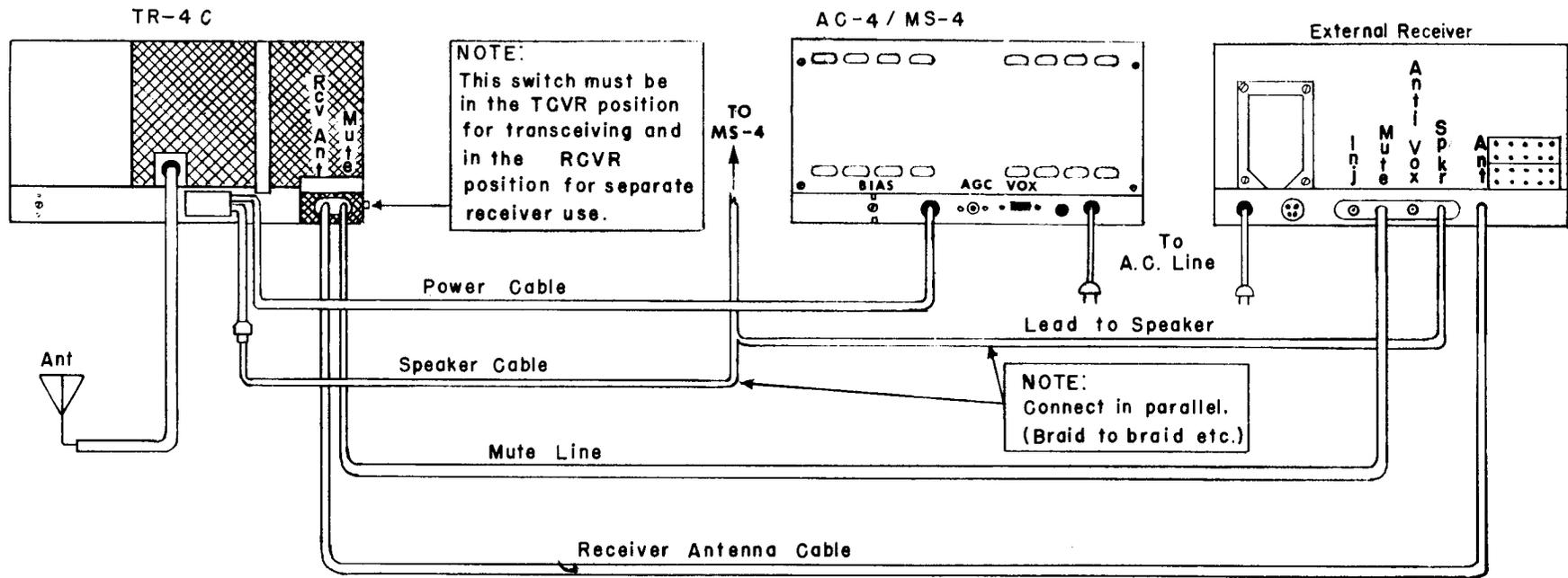
Figure 2-9. Connecting an External Receiver
