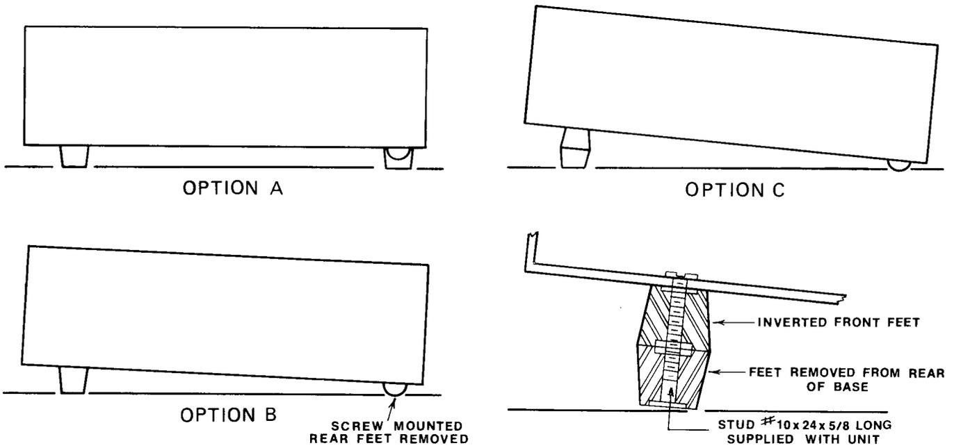
Figure 2-5. Viewing Angle Options in a Stationary Installation
