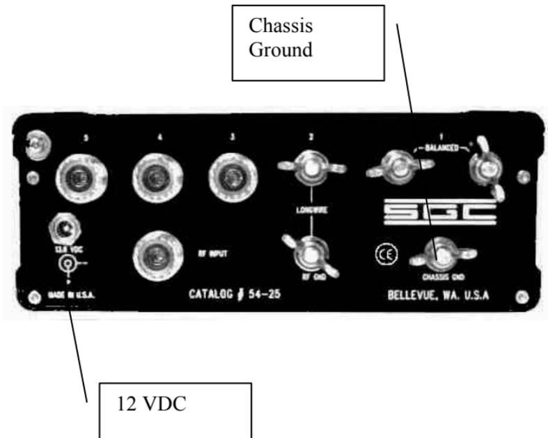
The MAC-200 has a miniature power input jack on the back panel. Any voltage from 10 to 18.5 VDC is suitable for operation. Average current draw will be approximately 230 milliamps. The MAC-200 should be powered from the same power source used to supply your transceiver to ensure that it is energized whenever the transceiver is in operation.
