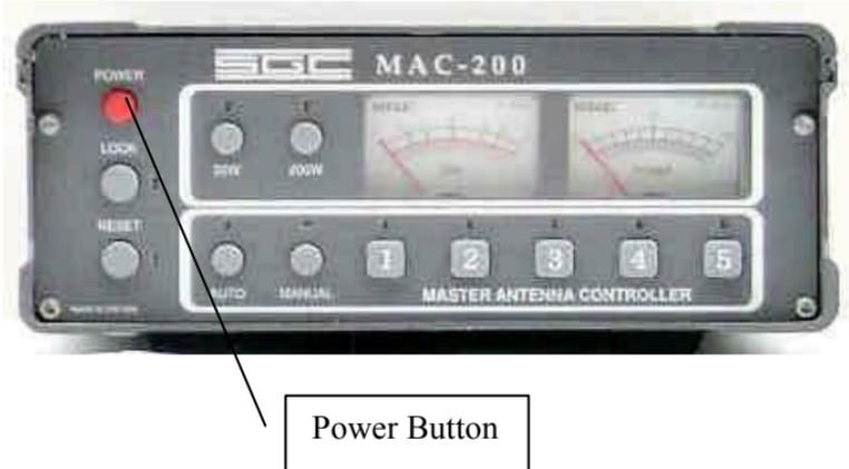
Momentarily press the Red Power button on the front panel to activate the MAC-200. You should see the LEDs behind the meter displays light up.
