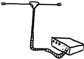
Balanced antennas can be connected to the balanced line connections on the back of the MAC-200.
