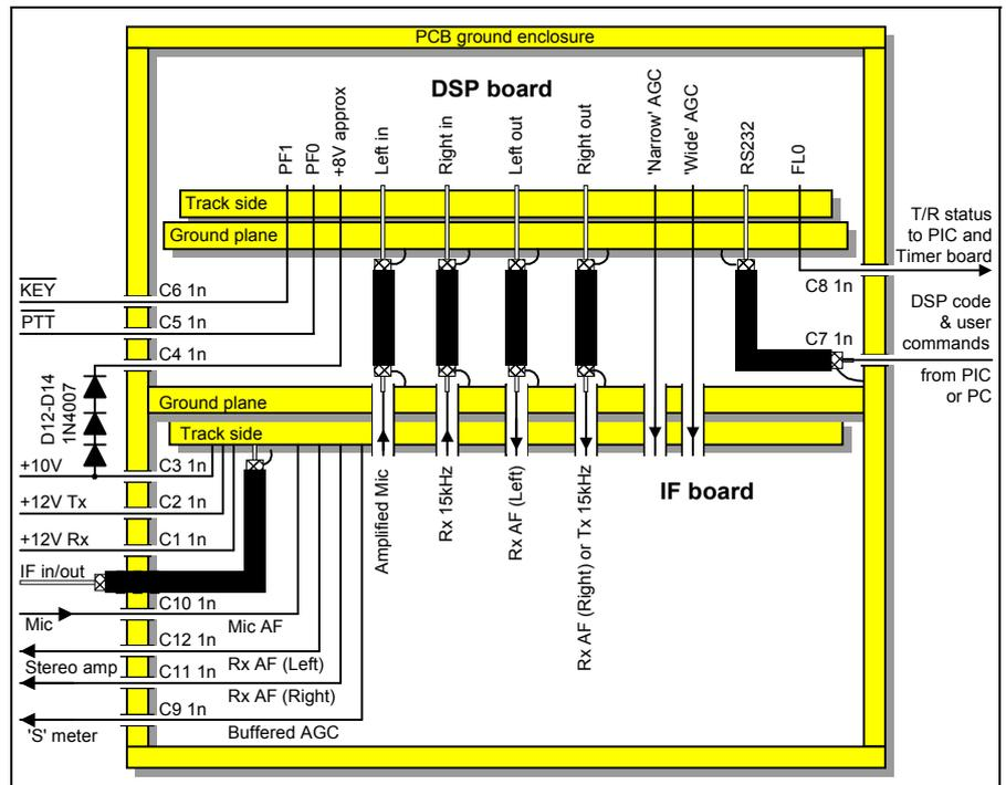
Fig 14: DSP sub-assembly. The IF board is bolted back-to-back to the DSP board using nuts, bolts and spacers. Both their groundplanes form a screen to isolate the two halves of the box. Feedthrough capacitors are used to route between the two halves of the box - and to the rest of the transceiver. C11 and C12 may be replaced with a stereo jack socket.
