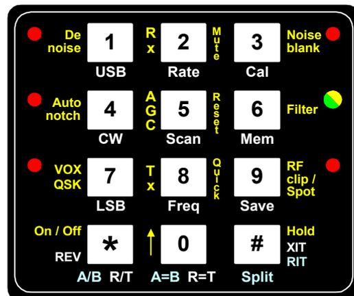
Fig 30: Keypad allocations and corresponding status LEDs. This is to scale and may be used as a keypad overlay. Note that this reflects recent developments.
