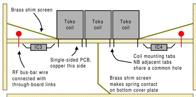
Fig 41: Cross-section of band-pass filter enclosure. The main board is single-sided with critical incremental screening on the top provided by brass shim. The same material is used to form a central spine shield running up the middle of the filters in the lower compartment. It is bent over to make spring contact with a bottom cover plate - made from PCB stock.
