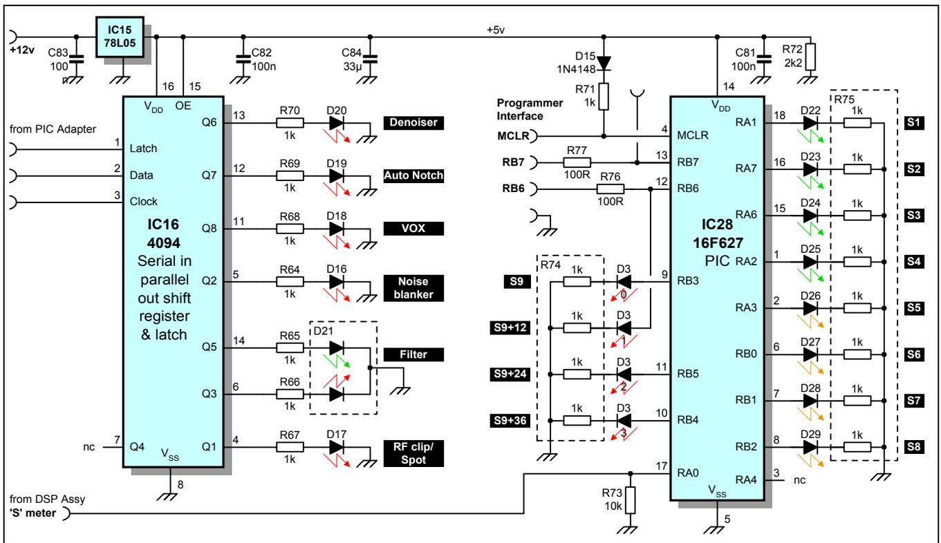
Fig 20: Status board circuit diagram. The status LEDs and driver are functionally unrelated to the 'S' meter LEDs and driver but they are co-located around the keypad. Not shown here are some merely passive tracks which are used to make off the 7-way ribbon cable to the keypad. The connector shown on RB7 is for future development only.
