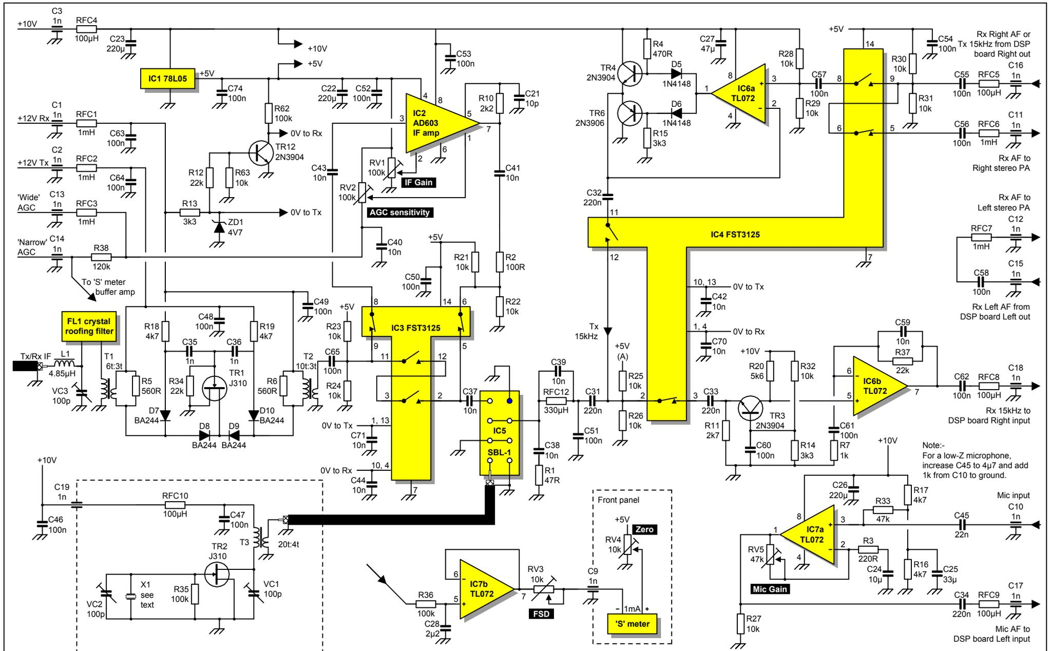
Fig 11: IF board circuit diagram. Takes an HF IF feed from a typical bi-directional mixer and post-mix amp and translates it to/from 15kHz. This board mounts back-to-back with the DSP board. All components are mounted on the track side except for the crystal filter FL1 and the SBL-1. The roofing filter is your choice and X1 must correspond. The switches in the receive path are shown as closed for illustration purposes only.
