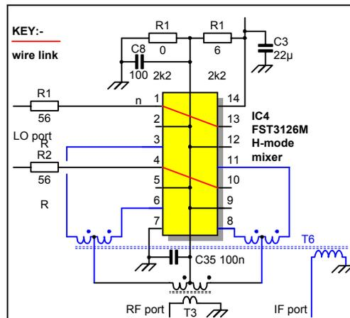
**Fig 37: Two-transformer H-mode mixer by I7SWX.** Details of transformer T6 (which replaces T4 and T5) will be provided next month. It is wound on the same ferrite as the other transformers.
