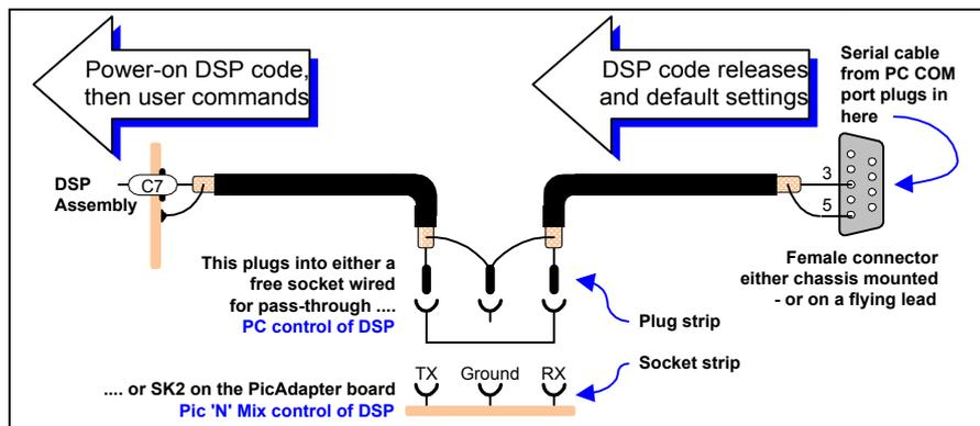
Fig 18: RS232 connections. This can be made up as one composite loom - or as two separate leads.
