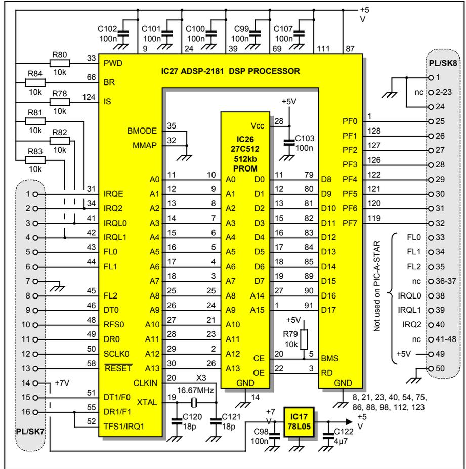
Fig 7: Processor daughter board circuit diagram. IC27 may be a KS-130 or KS-160 processor but in any event, the slower KS-130 device is assumed. To retain compatibility with EZLITE, the unused or unconnected lines on PL/SK8 are available on the mother board for non-STAR applications.
