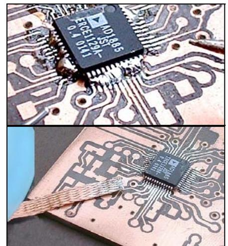
**CODEC chip before and after desoldering. Do not panic, it works!**
