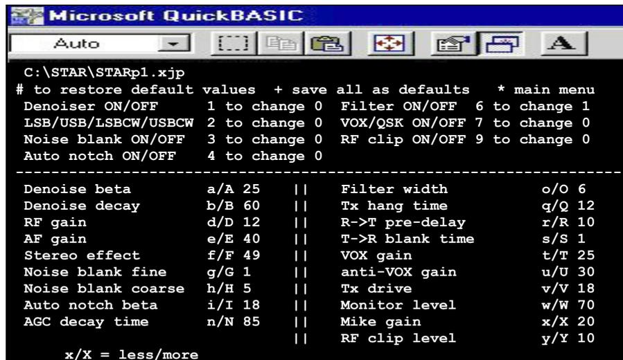
Fig 15: The PC screen running under *QBASIC*. Illustrated are the STAR parameters for the SSB mode. This has since been revised in appearance.
