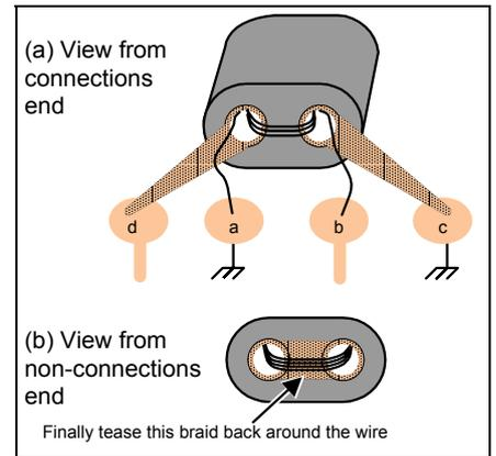
Fig 40: Transformer T1 detail. The pad designations correspond to those of fig 34.
