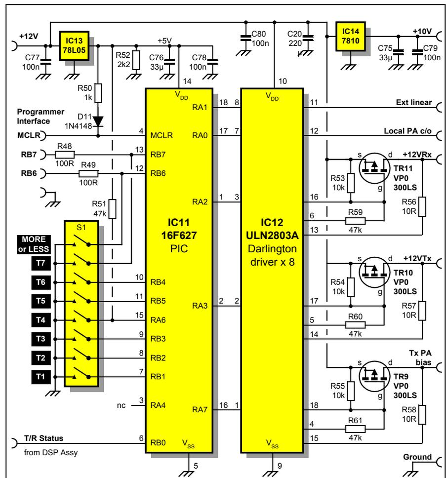
Fig 4: Timer board circuit diagram. This provides timed transitions between transmit and receive - in both directions. Sw1 allows you to set up the timing for your installation - and covers the range from slow relay-based RF T/R switching through to solid-state QSK.
