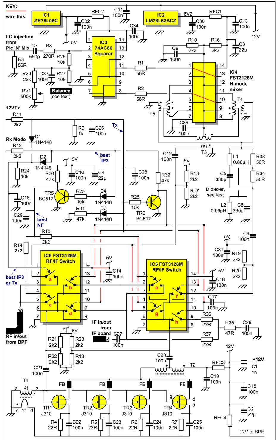
**Fig 34: Dynamically configurable H-mode mixer - and quad J310 amplifier, better known as the 'Magic Roundabout'. The 'Rx Mode' line is set to +5V ie logic '1' for best intercept (IP3) - or to logic '0' for best noise figure (NF). 12VTx - when taken to +12V - selects the transmit configuration. The mixer requires fundamental frequency injection between -10 and +10dBm.**
