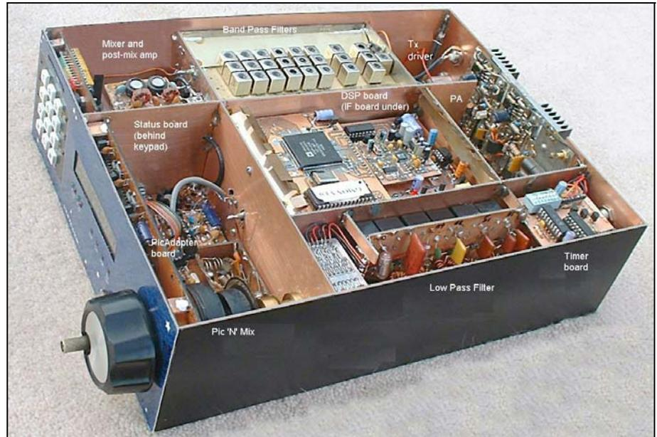
G3XJP's STAR built in a PCB enclosure - shown with all compartment cover-plates removed. The overall dimensions of the case are 310mm deep by 240mm wide by 85mm high. This generous size allows good *in situ* access to all the boards.
