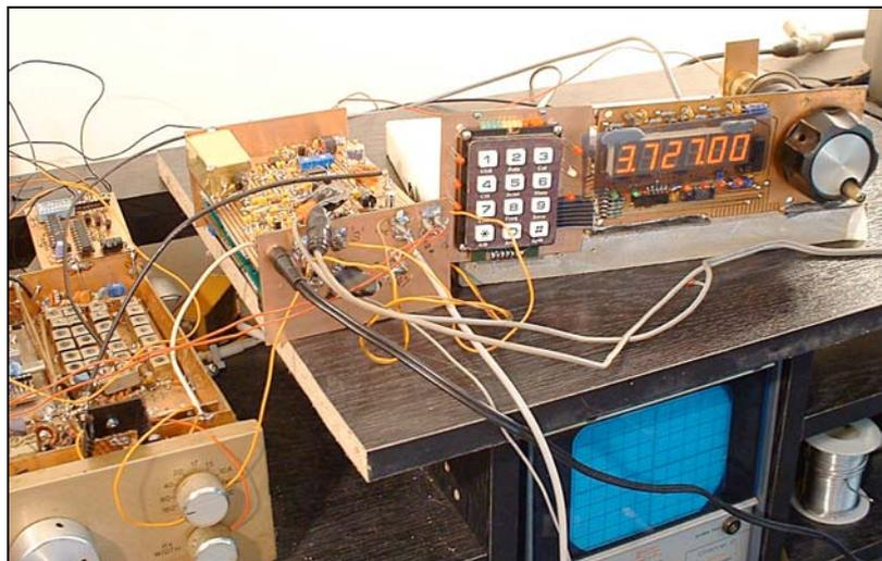
Early integration testing. Bottom left is my Third Method transceiver (borrowed front-end and PA), top right is Pic 'N Mix DDS still on its original breadboard (injection and controls) - and in the middle is the new DSP module under development. Note that Pic 'N Mix provides *all* the transceiver controls, leading to a clean and compact front panel.
