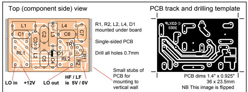
**Fig 28: Injection filter component layout and PCB.**
