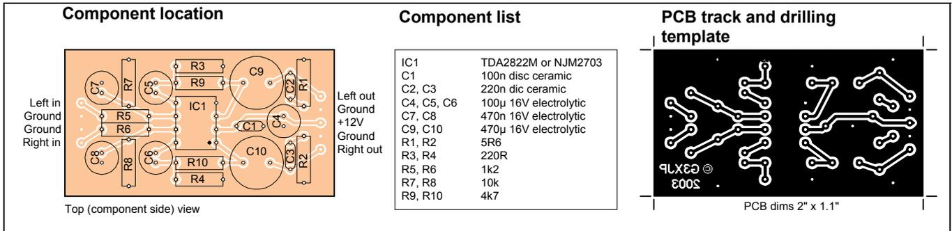
**Fig 22: Double-sided stereo amplifier PCB.** This is a 'conventional' board with components mounted on the top, the track underneath. The component side is completely unetched. No connectors are specified, but the relevant pads have a 0.1" pitch.
