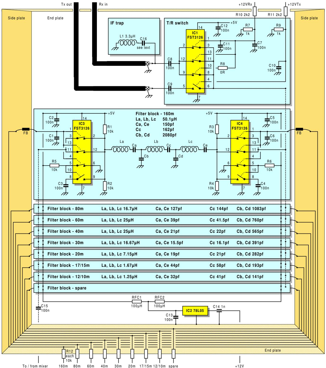
Fig 42: Band-pass filters circuit diagram and mechanical overview. All the filters have identical circuit diagrams. A band-select line is set to +5V to engage a filter block and to 0v to isolate it. This is compatible with direct interfacing to the Pic 'N' Mix band-select outputs. These lines are deliberately routed around the side-plates and *not* across the filter. For illustration, the 160m filter is shown 'on' and the T/R switch is 'on receive'.
