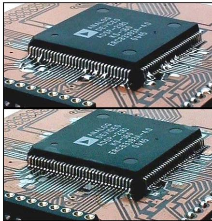
**Processor chip before and after removing excess solder. The target time to mount this 128-pin chip and clean up is 15 minutes.**
