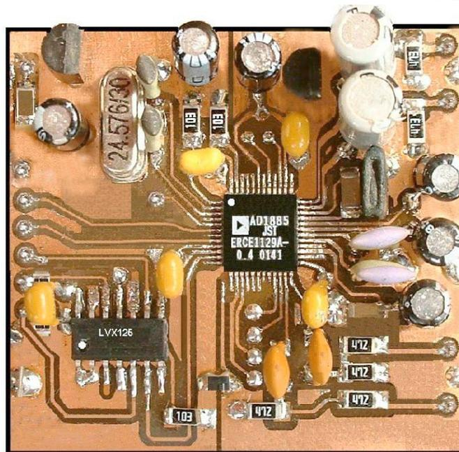
The completed CODEC board, illustrating the quality of PCB production available (0.2mm wide tracks at 0.5mm spacing) - using domestic kitchen resources. The CODEC chip is 7mm square.
