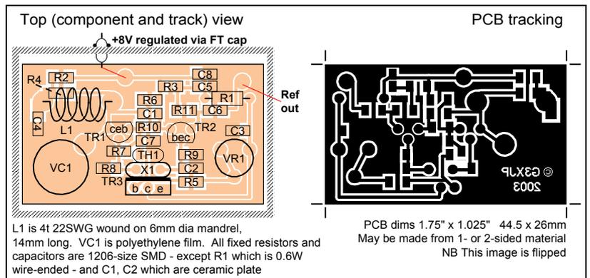
**Fig 29: Reference oscillator component layout and PCB.**
