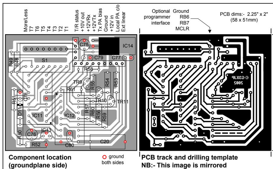
Fig 5: Timer board PCB - with the component side unetched. Countersink the ungrounded holes on the component side. The input/output connector (if any) is not specified, but is 0.1" pitch. I used SIL plug/socket strip for this - and all other arbitrary connectors.
