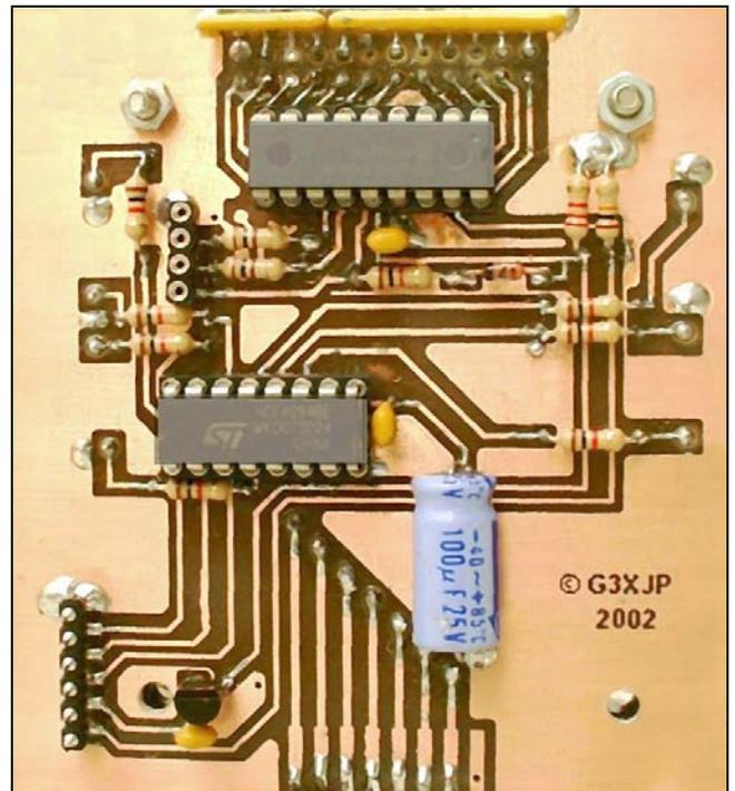
The Status board, viewed from rear. All the components are surface-mounted on this side of the board. The bottom row of connectors carry short links to the keypad.
