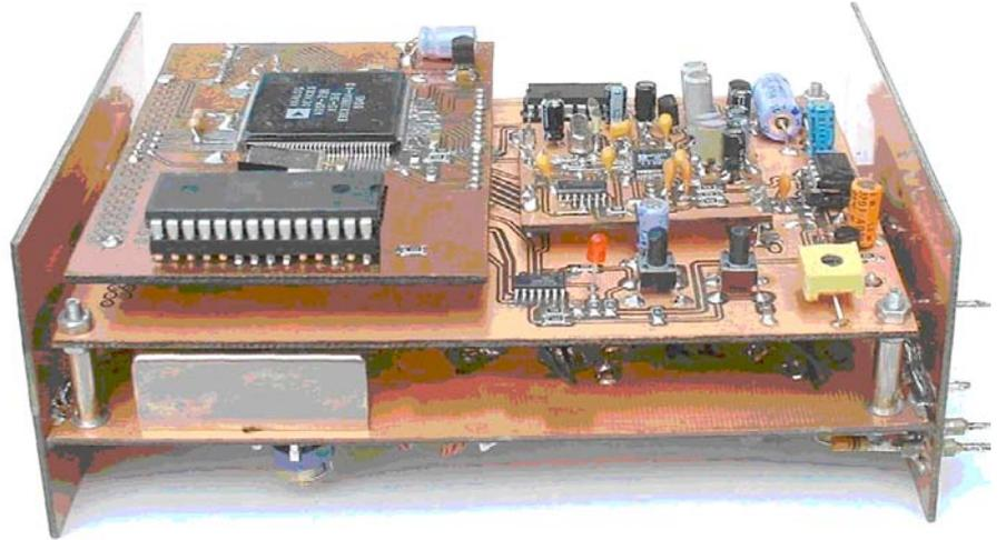
The DSP assembly. That is, the DSP mother board with CODEC and Processor daughter boards - mounted back-to-back with the IF board in its enclosure. The top, bottom and side screening panels are not fitted until after final test.
