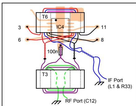
Fig 39: Details of T6 / T3 connections to each other and to IC4. This is not strictly to scale, but does show the correct relative positioning of the components. T6 and T3 will end up separated by about 6mm in practice.
