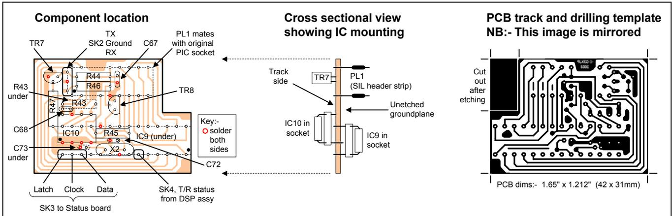
**Fig 23: Double-sided PicAdapter board PCB.** The cut-out is to give access to the existing programming socket. IC10 and IC9 should definitely be mounted in sockets. To achieve the clearance height required you may need to first fit an extra 18-pin socket into the existing Pic 'N' Mix socket - as a spacer. SIL plugs / sockets are used for the remaining leads - with the sockets soldered directly to the track.
