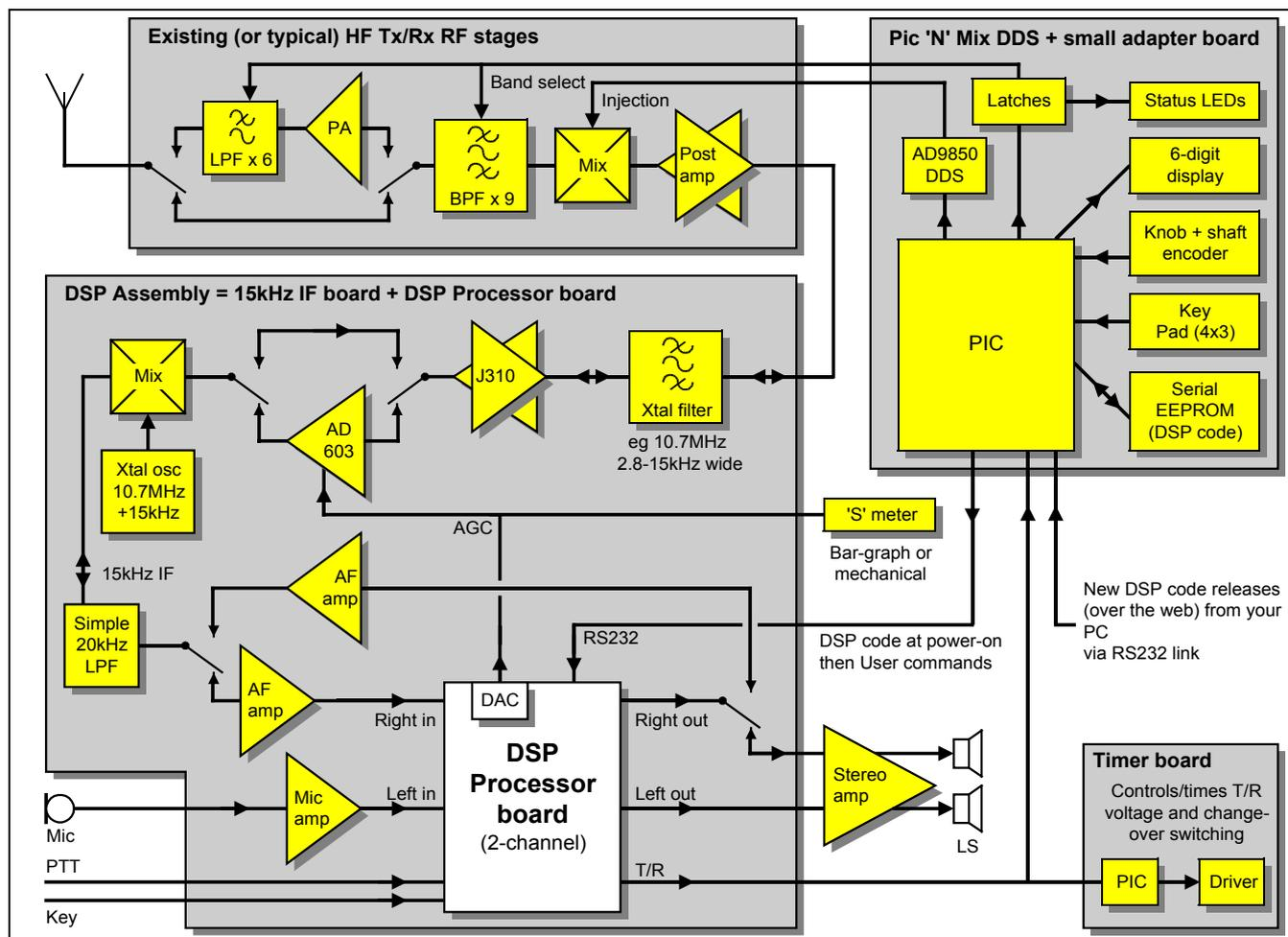
Fig 1: A typical transceiver incorporating PIC-A-STAR at a final IF of 15kHz. See text for a discussion of the major hardware elements.
