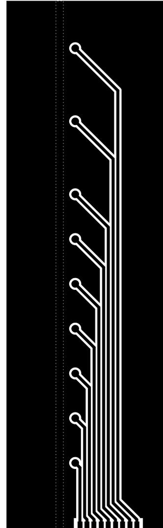
Drill these holes for tight fit on 1206 resistors
