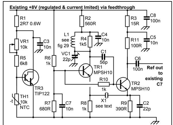
**Fig 27: Butler oscillator for either 5<sup>th</sup> or 7<sup>th</sup> overtone operation - with crystal temperature control.**
