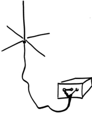
A vertical antenna may be connected to the SG-211 in a number of ways. Vertical antennas require an RF Ground system to function properly, but this may be incorporated into the design of the antenna itself.
