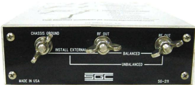
Optimum use of the SG-211 Smarttuner is to put it directly at the antenna feed point. This may require enclosing it in a waterproof enclosure to protect it from the weather. Either a balanced or an unbalanced antenna can be connected directly to the wing nuts provided on the back of the coupler.
