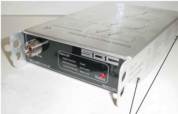
Two Cover Screws on each side, none on front and back
