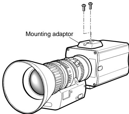
2. Fix the camera mounting base, pan/tilt unit, and tripod securely in the screw hole (1/4-20UNC) of the camera mounting adaptor.
